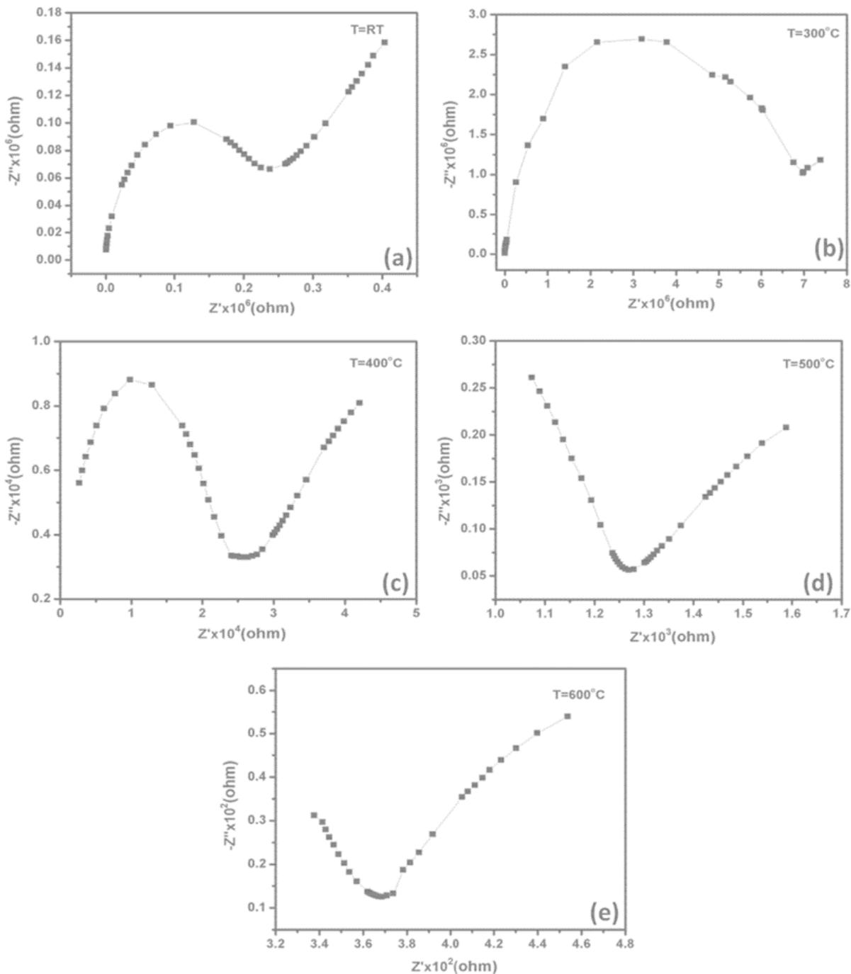
**Fig 8:** (a-e) Impedance curves obtained on sintered circular compacts of Ce<sub>0.9</sub>Gd<sub>0.1</sub>O<sub>2-δ</sub> at different temperatures
