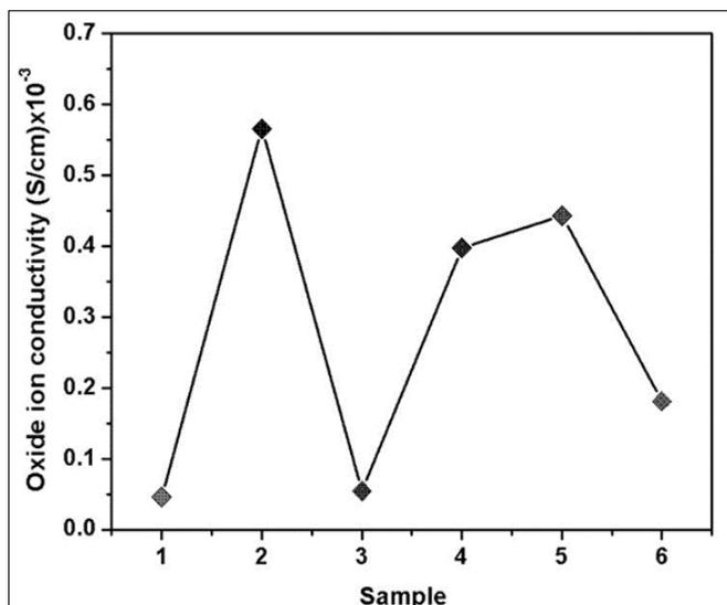
**Fig 10:** Curve obtained from conductivity values at 600 °C for different Compositions of nanocrystalline electrolyte powders
