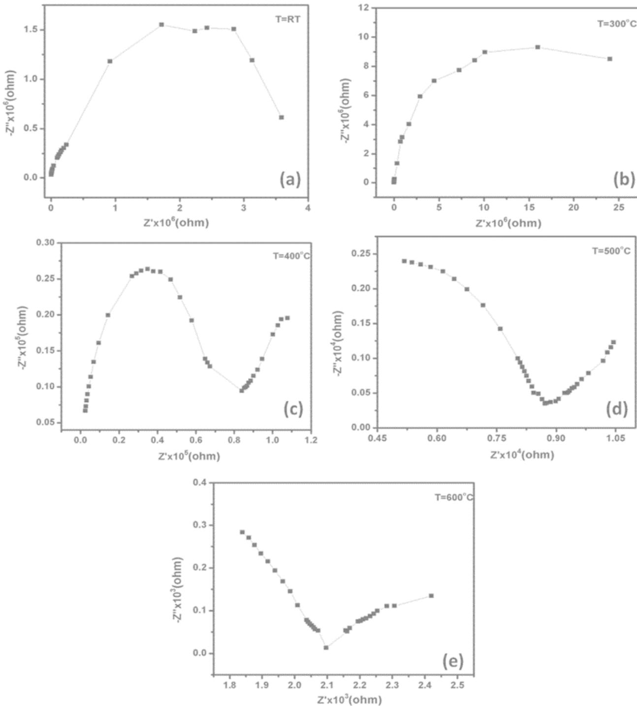
**Fig 6:** (a-e) Impedance curves obtained on sintered circular compacts of  $Ce_{0.9}Gd_{0.1}O_{2-\delta} - Ce_{0.9}Sm_{0.1}O_{2-\delta}$  at different temperatures
