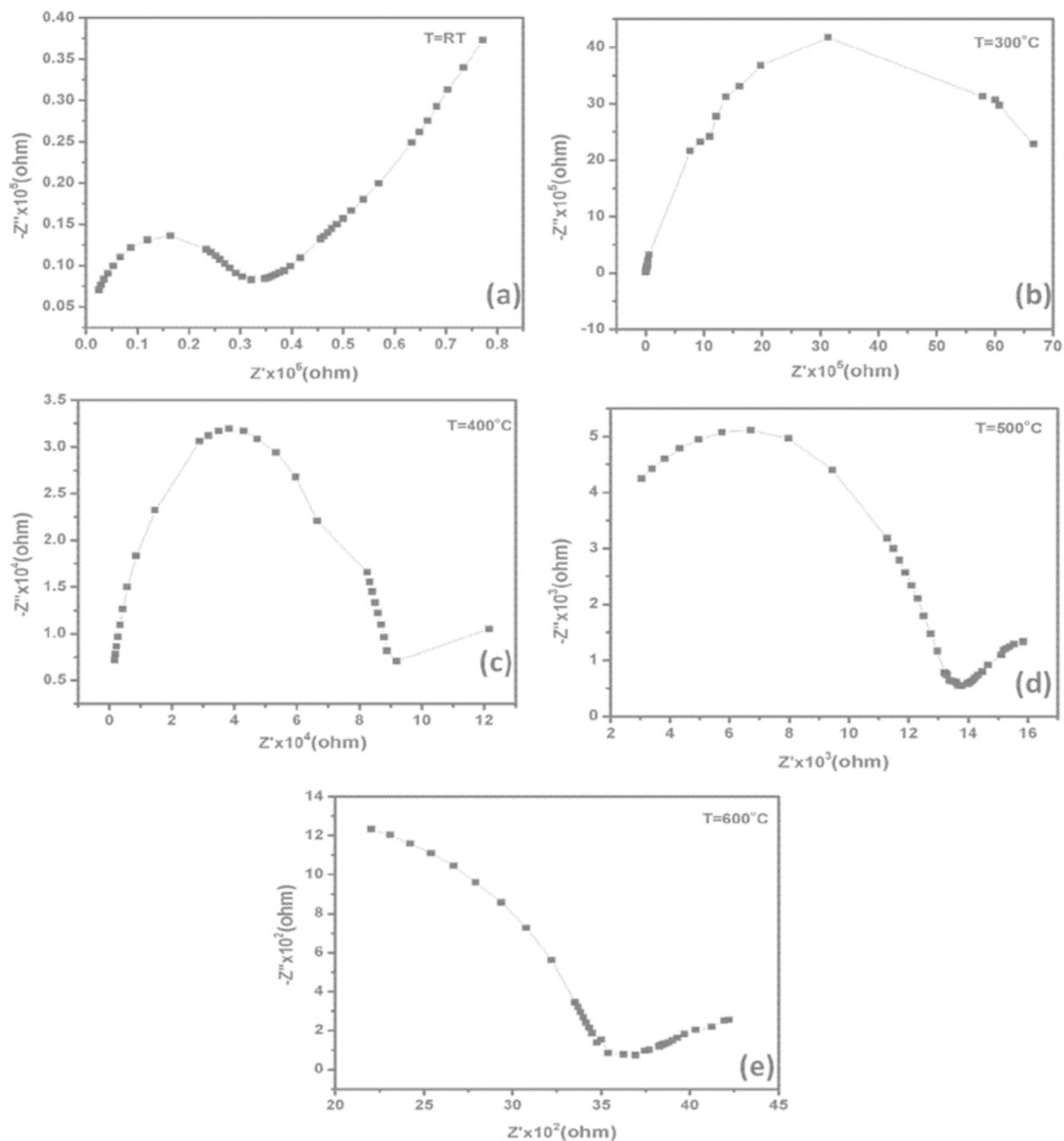
**Fig 4:** (a-e) Impedance curves obtained on sintered circular compacts of  $\text{Ce}_{0.9}\text{Gd}_{0.1}\text{O}_{2-\delta}$  -  $\text{Ce}_{0.9}\text{Y}_{0.1}\text{O}_{2-\delta}$  at different temperatures.
