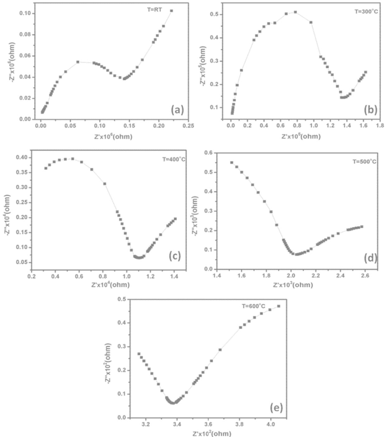
**Fig 5:** (a-e) Impedance curves obtained on sintered circular compacts of  $Ce_{0.8}Gd_{0.2}O_{2-\delta}-Ce_{0.8}Y_{0.2}O_{2-\delta}$  at different temperatures
