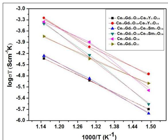
**Fig 11:** Arrhenius linear relationship plot obtained on nanocrystalline ceramic composite oxide pellets.
