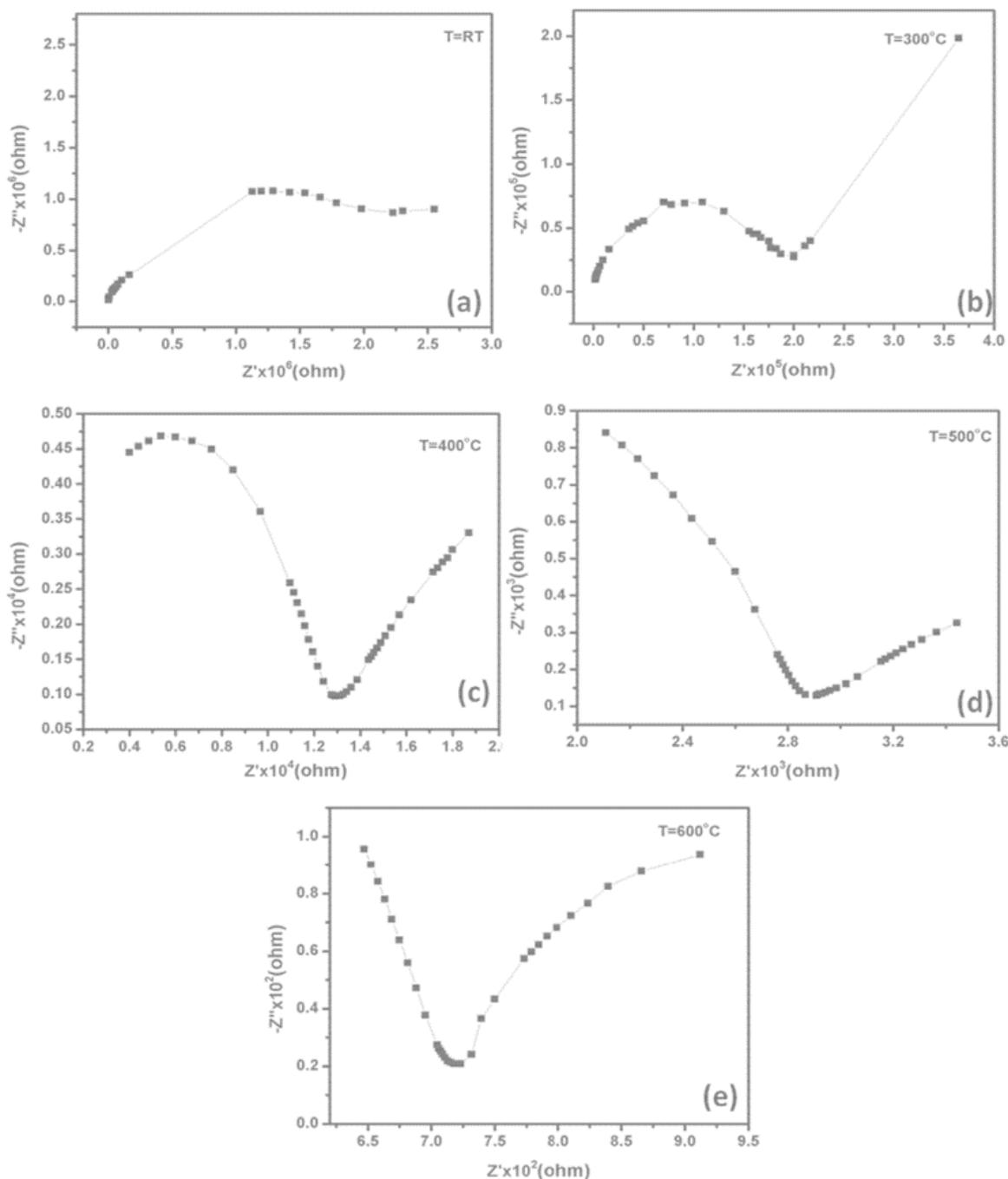
**Fig 9:** (a-e) Impedance curves obtained on sintered circular compacts of  $Ce_{0.8}Gd_{0.2}O_{2-\delta}$  at different temperatures
