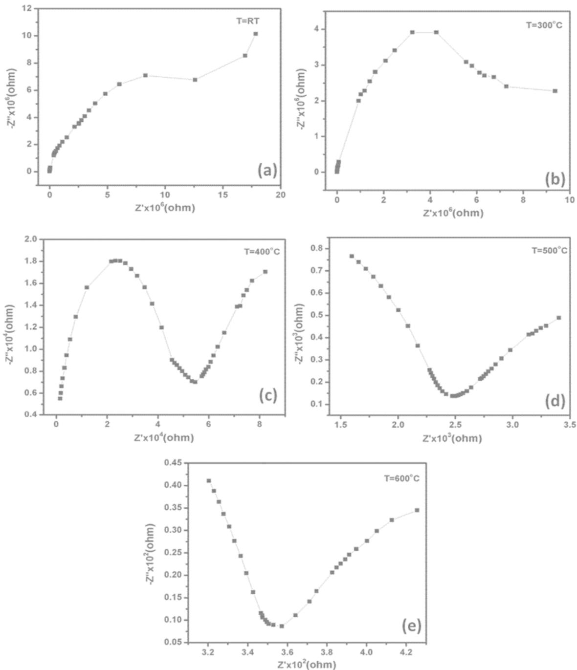
**Fig 7:** (a-e) Impedance curves obtained on sintered circular compacts of  $Ce_{0.8}Gd_{0.2}O_{2-\delta} - Ce_{0.8}Sm_{0.2}O_{2-\delta}$  at different temperatures
