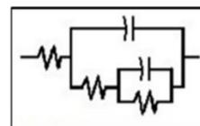
**Fig 3:** Equivalent circuit, used to fit measurement data obtained on doped ceria nanocomposite ceramic oxide pellets
