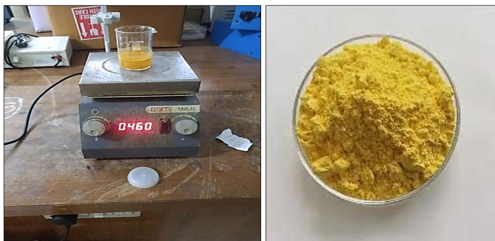
Step 2: Reaction of substituted 2-aminothiazole with Cyanuric chloride
