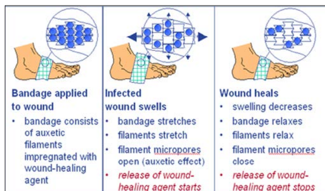
Functional Principle of Smart Bandage
